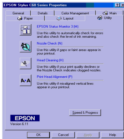
Figure 6-2. Head cleaning function in the printer driver utility
